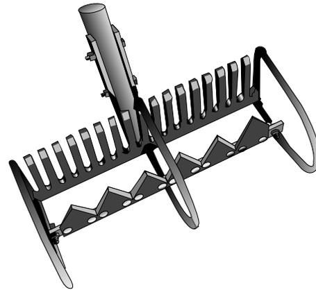
**Figure 4.** *Rockweed cutter rake.*
