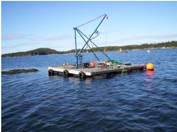
**Figure 6.** *Bagging floating platform unit.*
